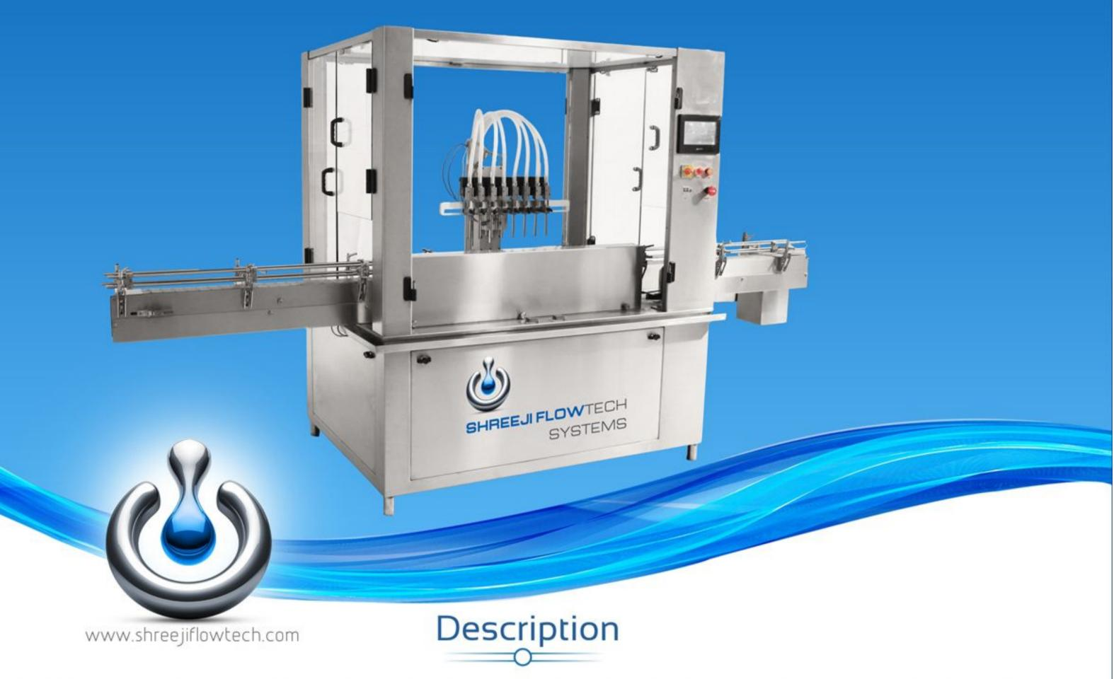
Servo Continuous motion & pneumatic diving nozzle based Gear Pump/Flow Meter filling machine offers flexibility for wide range of liquids with ease of simply. Gear pump fillers are positive displacement pumps with self-priming features. Pumps can fill minimum to maximum fill volume without any mechanical setting by HMI such as a flow meter. Gear Pump filling is a cheaper option of flow meter filling.
